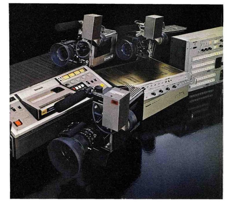
back beam control, the AK-760 has the necessary beam current to stabilize scene highlights to the point where comet tailing is greatly reduced.
